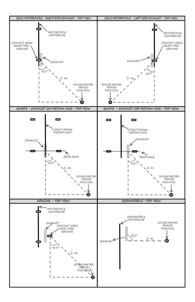
The sound level for engines with more than one silencer will be measured on each exhaust end.
